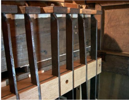
**Figure 35. Stop levers. The single pivot rod sits in a channel without fixings.**
