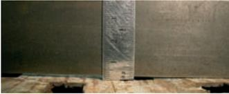
Figure 39. Measuring the distortion in the windchest table.
