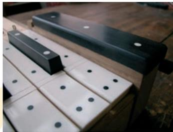
Figure 31. Pedal pull-down action assembly.
