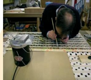
Figure 38. Glueing discs for levelling the table.
