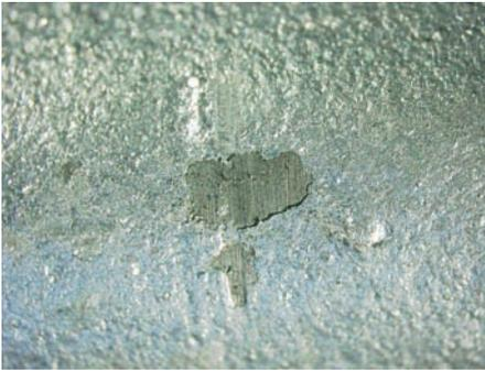
**Figure 2:** Area of organ pipe showing silver paint on metal surface. Sample OP4 removed from edge of damage.
