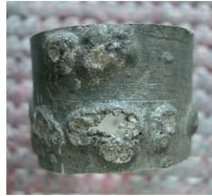
**Figures 75-76. Corroded pipe during repair.**
