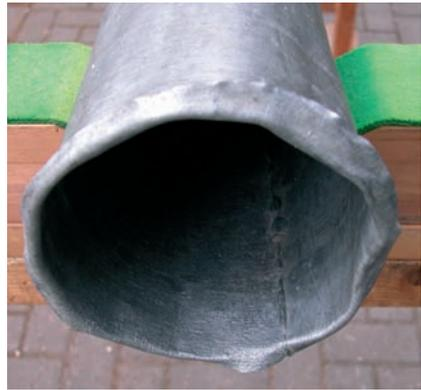
**Figure 63.** The end of the Trompeta Real C resonator, showing the marks of casting on cloth.
