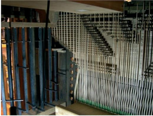
**Figure 32. Roller board and stop action.**
