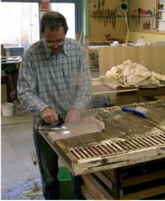
Figure 36. Removing sheepskin from the underside of the windchest.
