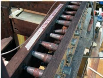
Figure 54. Trompeta Magna boots being fitted into the toeboard.
