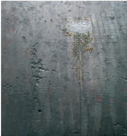
**Figure 62.** The inside of a front pipe, showing signs of sand casting.
